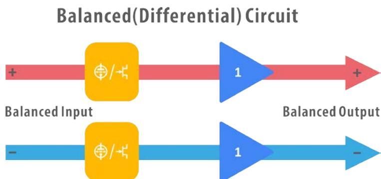
In detail: The Pro iCAN circuit is fully-balanced with completely equal circuit sections for Positive (Hot) and Negative (Cold) signal phase of each channel. The Volume control has 6-Decks, two decks each control the volume of one channel, and the other two decks are used for monitoring the volume control operation. This exceptional volume control potentiometer is custom made for iFi by ALPS Japan and has no parallel from other makers.
